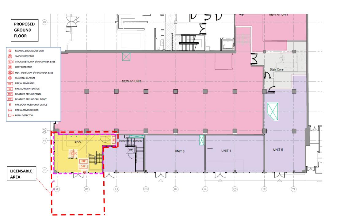
MANUAL BREAKGLASS UNIT SMOKE DETECTOR **PROPOSED** SMOKE DETECTOR c/w SOUNDER BASE **FIRST** HEAT DETECTOR **FLOOR** (h) HEAT DETECTOR c/w SOUNDER BASE FLASHING BEACON FIRE ALARM PANEL FIRE ALARM INTERFACE DISABLED REFUGE PANEL DCP DISABLED REFUGE CALL POINT (0) FIRE DOOR HOLD OPEN DEVICE FIRE ALARM SOUNDER ■ BEAM DETECTOR KIOSK KIOSK KIOSK EVENT SPACE TO CINEMA (m) (2) BAR **LICENSABLE** BAR STORE **AREA** SERVER ООМ
